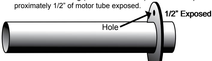
**IMPORTANT:** 38mm Aeropack Retainers require 3/8" of clean motor tube aft of the centering ring to mount. Adjust step 4 appropriately if you are using this retainer.
