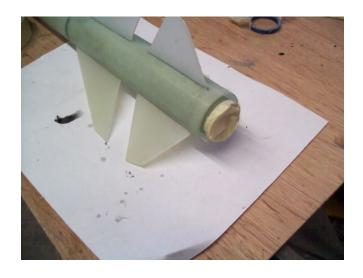
Prop up the airframe in the vertical position to hold steady while filling with 2-part foam.
