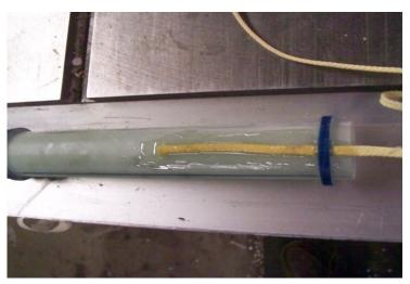
Then encapsulate the shock cord with epoxy. Epoxy top edge of CR to tube also. Don't get any inside or the motor won't fit!
