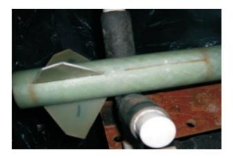
Then using cloths pin, chip clip, clamp, etc and a popsicle stick or other small straight edge, tack and align the upper 3 fins.
