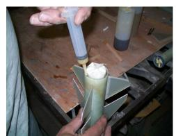
Let foam rise and set for 30-40 minutes. When cured it will be easy to scrape or cut off excess and sand residue.
