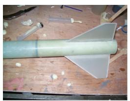
For the DarkStar do the bottom 3 fins first. Then use the clip, stick method described earlier to align upper and lower fins.
