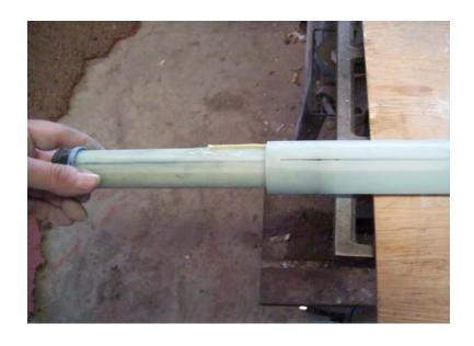
Wild Child :place bead of epoxy on bottom edge of fin, place into slot and align. Repeat for other 2 fins.
