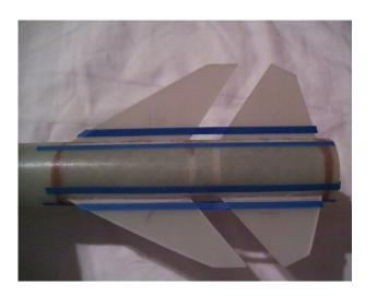
Place small amount of epoxy in grooves and smooth with rounded edge of stick. You may also thicken epoxy with filler if too runny. Either way, keep fillets tiny, you do not want to add unneeded weight! Epoxy darkened to make it easier to see.
