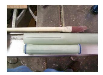
If using an Aero-pac for motor retention, first slide the rear CR on then epoxy the retainer on. Butt the CR up to front side of retainer and glue.
