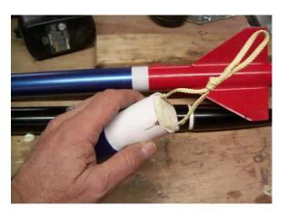
Glue ¼ in. diameter launch lugs ,¾ long, centered between the fins. One at rear of fincan & one just above front of fins. [Or rail buttons]
