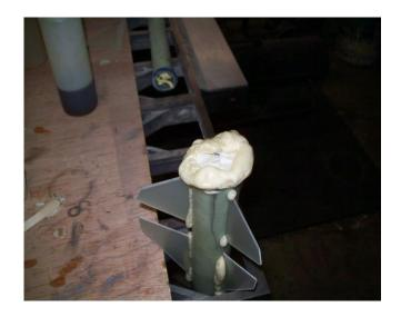
Finished fincan cleaned up and ready for next step. It is not necessary to use rear centering ring if foam is trimmed up neatly. Or you can install it if you wish. Just remove enough foam to get it in.
