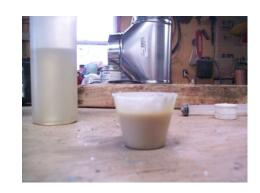
Cover tip, pour foam into syringe. Inject between fin & airframe. Repeat for other 2 fins.
