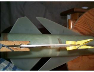
When using the CA to tack fins on: be careful NOT to get any on the rear CR! Don't tilt the airframe towards the rear CR so the superglue can run along a fin edge and glue the CR in! Use the Ca sparingly. Only need a drop or 2 per fin. This is just to hold the motor mount tube in position, then you pull out the rear centering ring, so you can pour in foam.
