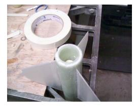
It takes 30ml [or cc, they are the same]of foam to fill the fincan, 15ml of part A and 15ml of part B. You must work fast, once you start mixing, the foam will begin to rise in 45 seconds to 1 minute depending on the temperature. Cut tip of syringe so you have a larger hole to work with if yours has a tiny one. Don't cut off too much, it still must fit between the airframe and motor mount tube.
