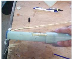
Make sure the rear CR is a loose fit so you can remove it with the tape tabs!
