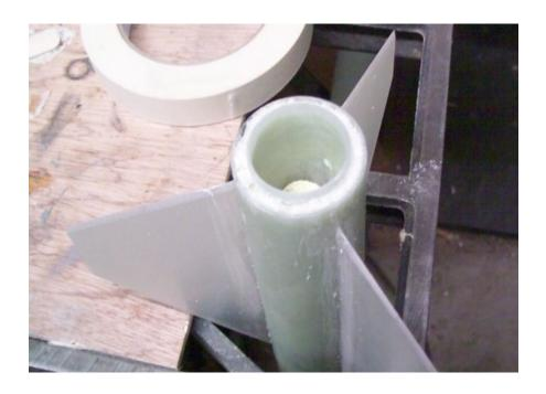
If using an Aero-Pac for motor retention, epoxy it on the motor mount tube now. They require ¼ in of exposed MM to glue on to. Sand any residue foam off MM and epoxy on.
