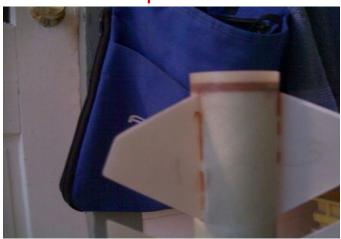
Tack remaining 2 fins. Align fins to insure straight flight. If experienced you may continue and tack upper fins and align. For those new to building split fin designs, let the rear set cure, then do the following:
