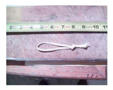
Tie overhand knot, insert loop through hole in NC bulkplate
