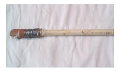
Tip: dowel or stick wrapped with the sandpaper taped on will make reaching inside to sand much easier.
