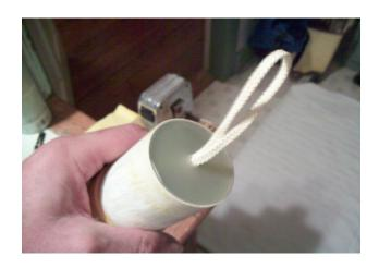
Install assembly into nose cone and epoxy into place. Sand bulkplate if needed, to fit into nose cone
