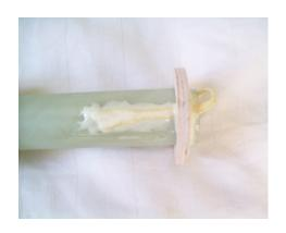
After filleting top of top CR ONLY, do NOT fillet bottom of top CR or fins won't fit between, then fillet inside of middle CR's only, and the outside if the rear CR. Remember NOT TO FILLET CR'S WHERE THE FINS WILL BE!
