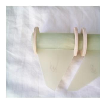
Slide MM assembly into position in the airframe. Make sure the kevlar shock cord is positioned **BETWEEN** the fin slots. The edges of all CR's should barely be visible at the ends of slots.
