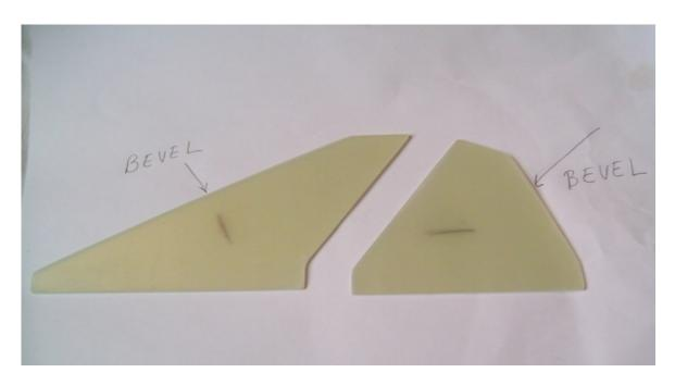
Fins do not come airfoiled [beveled], if you wish to do so, bevel or round over the top fin front edge and rear fin trailing edge with sandpaper. All other edges remain squared.
