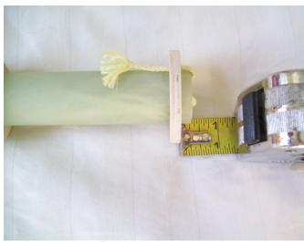
Slide remaining 3 CR's [centering rings]on the motor mount tube [MM]. Rear ¼ from edge of tube. Tack with CA. [superglue]
