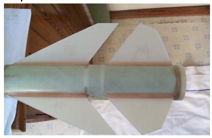
Drill 1/8 holes for rail guides. Try to hit bottom and top centering ring when mounting. This should be done before painting, so you can see the CR's through the glass. [I forgot to take pic, before I painted.]
