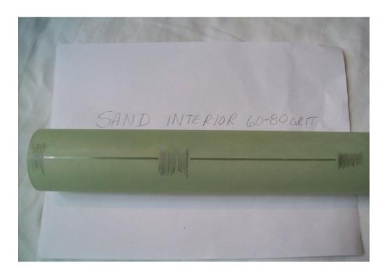
Tube is marked where the centering rings will be glued inside the airframe. Sand with 60-80 grit all around the circumference of the...... INTERIOR ..... of tube to promote glue adhesion.
