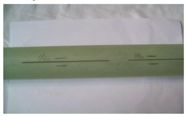
Sand the exterior of 29mm motor mount with 60-80 grit.
