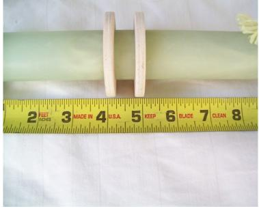
2<sup>nd</sup> from the rear 4in. from edge of MM tube. 3<sup>rd</sup> CR is 4 ¾ in. from rear of MM tube. Tack all CR's into place with CA and
