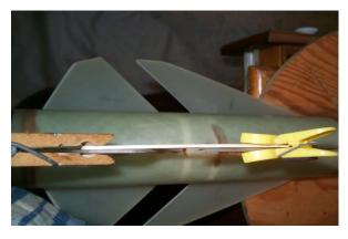
Use a popsicle stick or similar item and clothes pin, chip clip, clamp, etc, to hold upper fin in alignment with rear, after putting small bead of epoxy on root edge and inserting into airframe. Do remaining 2 fins. Stand tube on end and let cure.
