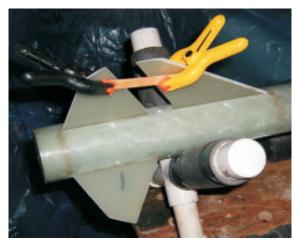
11) Sand your foils on the (3)forward fins. Install the upper fins, (1) at a time, coat the root edge with epoxy and install into the fin slot. You need to align the upper and lower fins with each other, use a popsicle or other flat stick and (2) small clamps to do this. Let cure and repeat on the remaining (2) fins.
