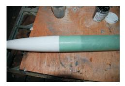
19) Mark the payload bay section with (2) holes, 180 degrees from each other and 1" for the top. Place the nosecone on payload and drill one 1/16th inch hole and then install a shear pin, then drill the other ( great way to get perfect alignment ). Also drill just one 1/8" hole in the middle of the payload bay section for Venting.
