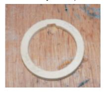
5) Notch the forward CR for attaching a shock cord using a 1/4 file, like above.
