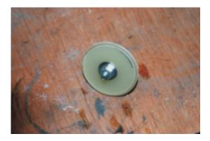
17) Glue a airframe bulkplate and coupler bulkplate together, using a eyebolt to line up and hold together. Repeat again for the second set and let cure.
