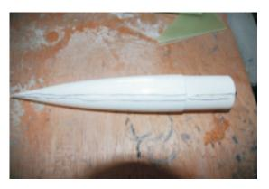
16) Sand or file exterior of nose cone smooth, removing all casting marks.
