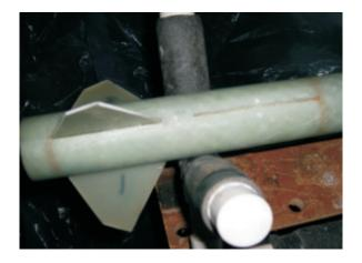
10) Now you'll install the Lower fins, (1) at a time, coat the root edge with epoxy and install into the fin slot, hold with tape if necessary in alignment, let cure. Then repeat with other (2) lower fins.
