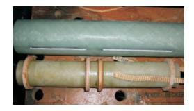
6) Glue the shock cord and forward CR into place on the motor tube. Let your motor assembly fully cure. After curing stuff the shock cord into the motor tube for safe keeping!
