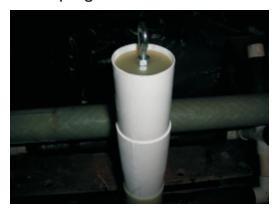
7) Sand or file the nosecone bulk plate to fit the nosecone (Don't sand the nosecone) Attach the Eyebolt to the bulk plate and then glue into place, and let cure (try setting the nosecone upright in the upper airframe to cure) If any gap are left using filler in the Epoxy to fill gaps.
