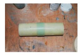
18) Glue the 1" switch band in the center of coupler, make sure there no glue on the edges and let cure. After curing, mark line ½" in for one side ( pick one ) all the way round the 1" band. Now mark (3) equally spaced cross mark on the switch band ( using a fin guide will help ). Using a 5/32 drill bit, drill those cross mark all the way thru the band and coupler ( these are for vent holes for the AV bay).
