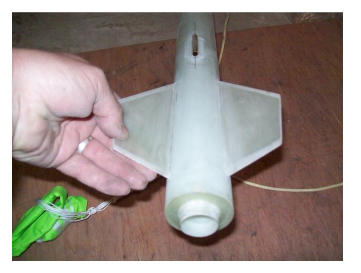
FILLET BOTH SIDES OF ALL 3 FINS TO AIRFRAME. SMALL FILLETS ARE ALL THAT ARE NEEDED. KEEP IT LIGHT.
