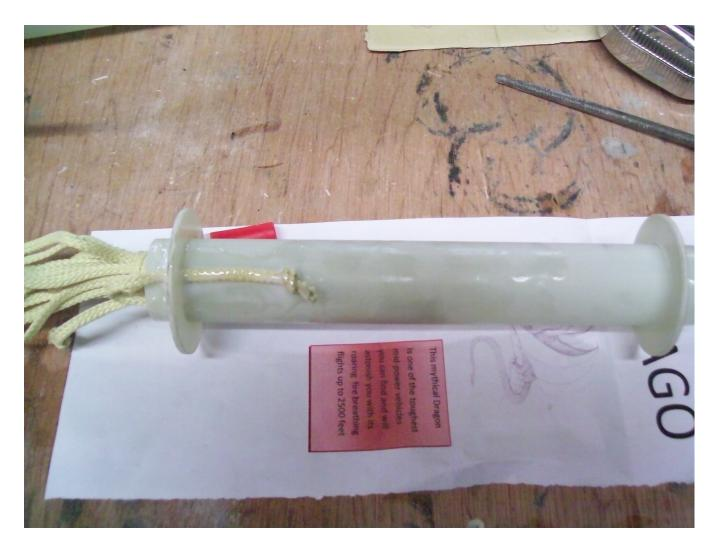
FILLET = GLUING A JOINT FROM ONE END TO THE OTHER, WHETHER STRAIGHT OR IN A CIRCLE. [THINK CAULKING A BATH TUB TO THE TILE.]
