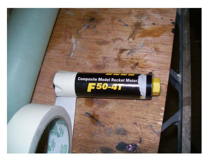
SLIDE MOTOR IN TUBE, BUTTING THE THRUST RING UP TO MOTOR MOUNT.
