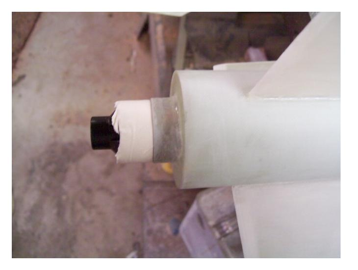
WRAP A COUPLE OF TURN OF TAPE AROUND THE THRUST RING AND MM. TUBE, SECURING YOUR MOTOR IN PLACE.
