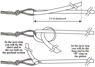
Prepare the parachute per the parachute instructions. Thread the shock cord through the loop you made in the parachute shroud lines and tie it using the knot illustrated on the left. Note that the chute should be attached to the shock cord at about the 1/3 point of the shock cord. Alternatively, you can tie the shock cord to a "kwik-link" and then attach the "kwik-link" to the loop in the shroud lines.
