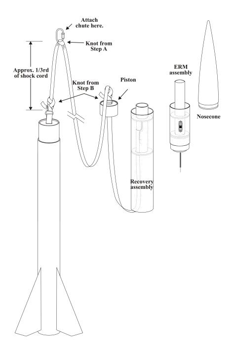
Slip the nosecone into position atop the ERM Section. Secure it in place using a minimum of 3 screws or rivets. Be sure to pre-drill the airframe when using screws.
