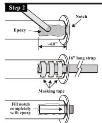
Spread a layer of epoxy about 1" wide and 4" long on the motor tube just below the notch in the upper centering ring. Slip one end of the 16" long strap through the notch in the centering ring. Pull through about 4" of this strap through the notch and press it firmly into the epoxy on the side of the motor tube. Hold the strap in place against the tube with masking tape until the epoxy cures. Remove the masking tape.
