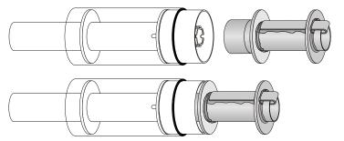
**A)** Make a mark on a stick at 3.0" so you can tell how deep the stick is in the airframe when spreading the epoxy. Spread a bead of epoxy around the inside circumference of the Fore Recovery Airframe 3.0" from the bottom of the airframe.
