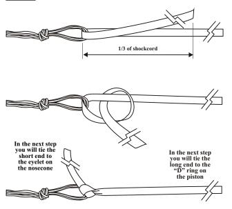
Prepare the parachute per the parachute instructions. Thread the shock cord through the loop you made in the parachute shroud lines and tie it using the knot illustrated on the left. Note that the chute should be attached to the shock cord at about the 1/3 point of the shock cord. Alternatively, you can tie the shock cord to a "kwik-link" and then attach the "kwik-link" to the loop in the shroud lines.
