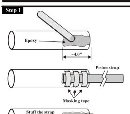
Spread a layer of epoxy about 1" wide and 4" long on the motor tube. Press 4" of the strap firmly into the epoxy on the side of the motor tube. Hold the strap in place against the tube with masking tape until the epoxy cures. Remove the masking tape. Stuff the free end of the strap into the motor tube to keep it out of the way for the next few steps.
