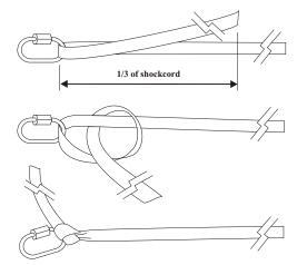
Thread the shock cord through the Kwik-Link and tie it using the knot illustrated on the left. Note that the Kwik-Link should be attached to the shock cord at about the 1/3 point of the shock cord.
