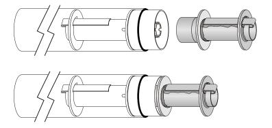
**A)** Make a mark on the stick at 3.0" so you can tell how deep the stick is in the airframe when spreading the epoxy. Using your extended epoxy applicator, spread a bead of epoxy around the inside circumference of the Fore Recovery Airframe 3.0" from the bottom of the airframe.
