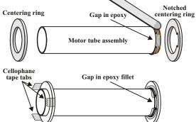
Spread a bead of epoxy around the circumference of the threaded adapter retainer leaving a 1" gap in the bead at the notch in the rib. Slip the notched centering ring over the threaded adapter retainer with the notch aligned with the gap in the epoxy bead. Be sure the notch in the ring remains clear of epoxy. Locate the ring against the rib and with the notches aligned. Allow the epoxy to
