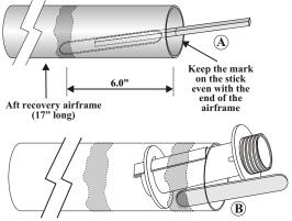
B) Push the altimeter mounting tube assembly about 2" into the aft recovery airframe. Spread another bead around the inside circumference about 1/2" from the end of the airframe. You can push the assembly from one side to the other to make it easier to reach with the epoxy applicator.
