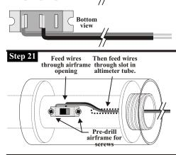
Strip about 1/4" of the insulation from the two wires and "tin" the exposed wires with a bit of solder to stiffen them. These wires will be attached to the power terminals of the altimeter.
