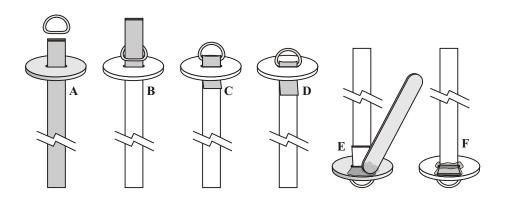
A) Pull the free end of the strap through the slot in the piston bulk plate.
