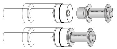
**A)** Make a mark on a stick at 3.0" so you can tell how deep the stick is in the airframe when spreading the epoxy. Spread a bead of epoxy around the inside circumference of the Fore Recovery Airframe 3.0" from the bottom of the airframe.
