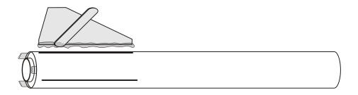
C) Using the tape as handles, gently pull the lower centering ring off the end of the rocket. Using a stick, apply an epoxy fillet to the fins at the motor mount tube and the inner airframe wall.
