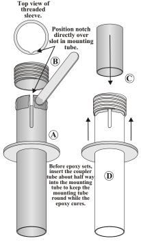
**A)** Slide the standard centering ring over the slotted mounting tube to the area below the slot.
