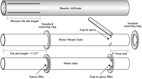
Measure the fin slot length on the booster airframe. Add 1-1/2" to this measurement. Make a mark on the motor tube at that distance. Epoxy one of the standard centering rings at this location. Apply a fillet to both sides of the ring.
