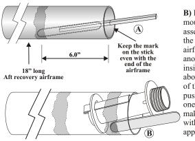
**B)** Push the altimeter mounting tube assembly about 2" into the aft recovery airframe. Spread another bead around the inside circumference about 1/2" from the end of the airframe. You can push the assembly from one side to the other to make it easier to reach with the epoxy applicator.
