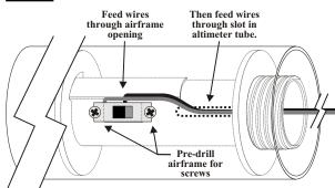
Feed the wire ends into the airframe opening, then through the slot in the altimeter tube and finally out through the end of the altimeter tube. Set the switch into the airframe hole (or stand-off), pre-drill the airframe for the mounting screws, and install the screws. Mark the airframe near the switch for the on-off positions.
