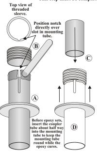
A) Slide the standard centering ring over the slotted mounting tube to the area below the slot.B) Spread a layer of epoxy around the slotted end of the tube. Keep the epoxy away from the slot. Slip the threaded sleeve over the tube making sure the small notch in the top of the threaded sleeve is aligned over the slot in the tube.
