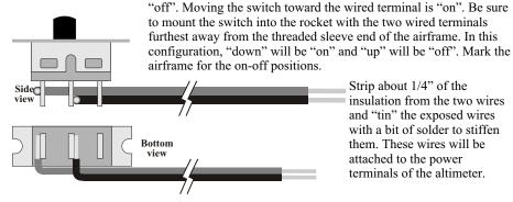
Strip about 1/4" of the insulation from the two wires and "tin" the exposed wires with a bit of solder to stiffen them. These wires will be attached to the power terminals of the altimeter.
