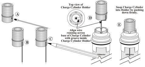
E) Determine the correct amount of FFFFg Black Powder to use for proper ejection using the chart below. Measure-out the Black Powder and pour it into the Charge Cylinder.F) Fill the remainder of the Charge Cylinder with a crumpled piece of flame-proof wadding to keep the Black Powder from moving about.
