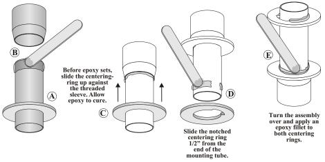
**D**) Spread a layer of epoxy around the circumference of the opposite end of the tube about 1/4" from the end. Leave a 1" gap in the epoxy. Push the notched centering ring onto the tube with the notch aligned with the gap in the epoxy. Position the ring 1/2" from the bottom. Allow the epoxy to cure.
