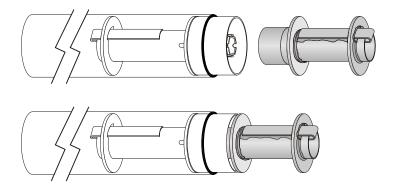
**A)** Make a mark on the stick at 3.0" so you can tell how deep the stick is in the airframe when spreading the epoxy. Using your extended epoxy applicator, spread a bead of epoxy around the inside circumference of the airframe 3.0" from the bottom of the airframe.
