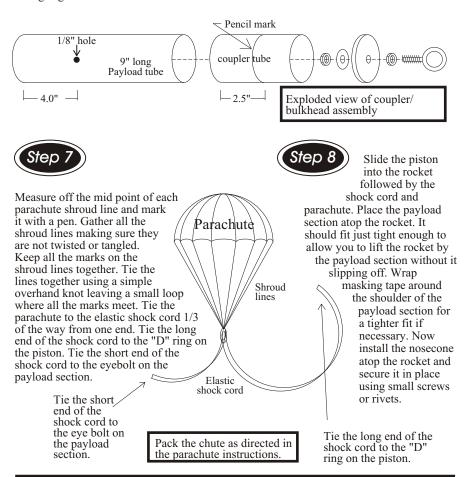
When tying the shock cord to the parachute and the "D" ring, loop the shock cord through twice then tie a double overhand knot. Pull the knot tight and leave 2-3 inches of excess cord after the knot.
