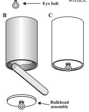
**B**) Spread a layer of epoxy around the inside circumference of the coupler to a depth of about 1/2". C) Push the bulkhead assembly into the coupler until it is about 1/4" past the edge. Allow the epoxy to set. **D**) Apply an epoxy fillet to both sides of the bulkhead. E) Draw a pencil mark at the midpoint of the coupler.
