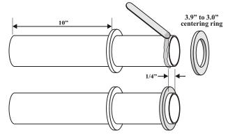
Spread a bead of epoxy around the circumference of the 3" recovery tube, 1/4" from the end nearest the ring previously installed. Slip the centering ring over the recovery tube. Locate the ring 1/4" from the end of the recovery tube as shown and allow the epoxy to set. Apply an epoxy fillet to each side of the ring.
