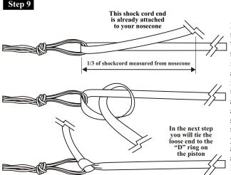
Prepare the parachute per the parachute instructions. Thread the shock cord through the loop you made in the parachute shroud lines and tie it using the knot illustrated on the left. Note that the chute should be attached to the shock cord at about the 1/3 point of the shock cord measured from the nosecone. Alternatively, you can tie the shock cord to a "kwik-link" and then attach the "kwik-link" to the loop in the shroud lines.
