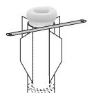
Grind or carve the foam below the end of the airframe until there is clearance for the centering ring. Remember that the motor tube must protrude 3/8" beyond the ring
