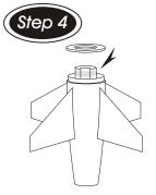
Apply a bead of epoxy near the top of the motor tube and slide the centering ring back into position over the motor tube. Turn the entire assembly upside-down so that the epoxy pools at the underside of the centering ring. Allow the epoxy to cure.
