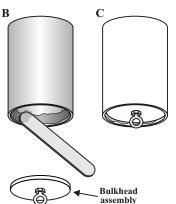
**B)** Spread a layer of epoxy around the inside circumference of the coupler to a depth of about 1/2".
