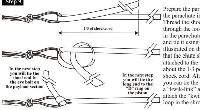
Prepare the parachute per the parachute instructions. Thread the shock cord through the loop you made in the parachute shroud lines and tie it using the knot illustrated on the left. Note that the chute should be attached to the shock cord at about the 1/3 point of the shock cord. Alternatively. you can tie the shock cord to a "kwik-link" and then attach the "kwik-link" to the loop in the shroud lines.
