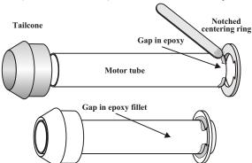
Spread a bead of epoxy around the circumference of one end of the centering ring motor tube leaving a 1" gap in the bead for the notch in the centering ring. Slip the notched centering ring over the motor tube with the notch aligned with the gap in the epoxy bead. Be sure the notch in the ring remains clear of epoxy. Locate the ring 1/2" from the end of the motor tube and allow the epoxy to set. Apply an epoxy fillet to each side of the ring still keeping the notch clear.
