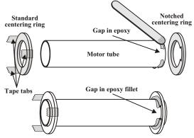
Spread a bead of epoxy around the circumference of one end of the motor tube leaving a 1" gap in the bead for the notch in the centering ring. Slip the notched centering ring over the motor tube with the notch aligned with the gap in the epoxy bead. Be sure the notch in the ring remains clear of epoxy. Locate the ring 1/2" from the end of the motor tube and allow the epoxy to set. Apply an epoxy fillet to each side of the ring still keeping the notch clear.
