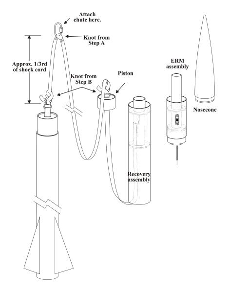
Slip the nosecone into position atop the ERM Section. Secure it in place using a minimum of 3 screws or rivets. Be sure to pre-drill the airframe when using screws.
