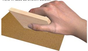
■ 4. Round all the edges of each fin, except the root edges. Leave them flat. Repeat for all eight fins. The root edges will be glued to the body tube.
