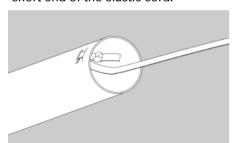
13. Apply a bead of glue inside the bottom of the insulating tube (away from the elastic cord.) Insert the engine mount into the insulating tube until it is recessed about 1/16" from the bottom of the top ring. Roll the assembly on a flat surface to make sure it is aligned properly.
