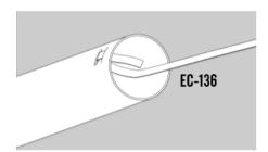
**12.** Tie an overhand knot in the short end of the elastic cord.
