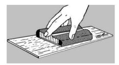
**3.** Stack all the fins in two groups. Line the groups up squarely and sand the fins back and forth over some fine sandpaper to get rid of the hold-in tabs as shown below. Do not sand enough to change the shape of the fins.
