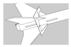
and the through-the-wall tabs of one of the two main wings and insert it into one of the double slots on the main body tube. Use the same method that you used to attach the small fins. The fin template can be used to check for alignment, but since the balsa is thicker, the slots will need to be enlarged slightly. Sighting from the top of the model will also work to align the fins.
