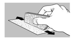
**4.** Round all leading edges and round or taper all trailing edges. Leave the tip and root edges flat.
