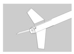
☐ 14. After the fin assembly is completely dry, run a small bead of glue along both sides of each finbody tube joint. Using your forefinger, smooth the glue into fillets.
