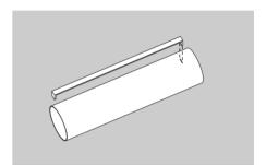
**7.** Apply a small bead of glue around the inside of the engine tube nearest the punched end. Slide the thrust ring (TR-7) into the tube and against the engine hook.
