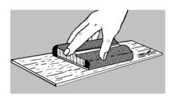
**3.** Stack all three fins in a group. Line the group up squarely and sand the fins back and forth over some fine sandpaper to get rid of the holdin tabs as shown below.
