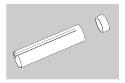
**8.** Slide the centering ring (CR-78L) over the engine tube until it is centered between the two ends. Apply a bead of glue around each end of the joint between the two tubes, keeping glue off the outside surface of the centering ring. Allow to dry completely.
