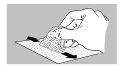
The fins and shrouds (conduits) are the most difficult task. Patience and careful sanding will provide a good scale shape for the fins. Begin by marking the centerline around all the fins. Place a fin inside the template (IKD-3T) as shown and use a felt-tip pen or soft pencil to place the mark. This will be used while sanding to keep the sides symmetrical.
