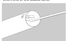
□ 13. Apply a bead of glue inside the bottom of the insulating tube (away from the elastic cord.) Insert the engine mount into the insulating tube until it is recessed about 1/16". Roll the assembly on a flat surface to make sure it is aligned properly.
