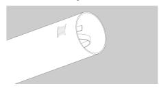
■ 16. Insert the insulating tube and engine mount assembly into the main body tube (ST-1095S3) until the lower centering ring is just outside the main body tube. Align the engine hook between two of the slots. Apply a heavy bead of glue around the top side of the lower centering ring.
