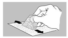
4. Round all the edges except the root edges of each fin. Do not sand the root edge or the tab will not contact the engine tube in a later step.
