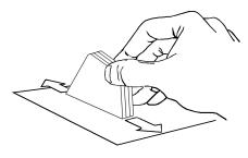
**3.** Round the leading and trailing edges of each fin. Leave the tip and root edges flat. Repeat for all three fins. The trailing edge can be sanded to a bevel for a more aerodynamic shape. The root edge will be glued to the body tube.
