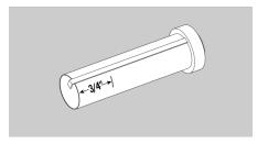
**9.** Slide the remaining centering ring (CR-710) over the engine tube until the mark is even with the bottom of the ring. Apply a bead of glue around both rings where they contact the engine tube. Keep glue off the outside edge of both rings. Allow the assembly to dry.
