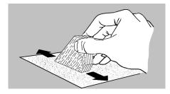
4. Round all the edges except the root edges of each fin. Do not sand the root edge or the tab will not contact the engine tube in a later
