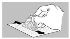
**4.** Round all the edges except the root edges of each fin. Do not sand the root edge or the tab will not contact the engine tube in a later step.
