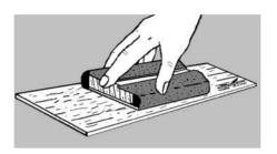
**3.** Stack all the fins in groups. Line the groups up squarely and sand the fins back and forth over some fine sandpaper to get rid of the hold-in tabs as shown below. Do not sand enough to change the shape of the fins.
