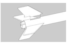
□ 19. As the fins are drying, use the laser-cut fin template to align the fins perpendicular to the main body tube. The template will work with three or four fins. Turn it until the three fins line up with the corresponding slots. Do not let any glue set with the template in place.
