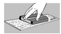
3. Stack all the fins in a group. Line the group up squarely and sand the fins back and forth over some fine sandpaper to get rid of the holdin tabs as shown below. Do not sand enough to change the shape of the
