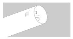
engine mount assembly into the main body tube (ST-10100S3) until the lower centering ring is just outside the main body tube. Align the engine hook between two of the slots. Apply a heavy bead of glue around the top side of the lower centering ring.
