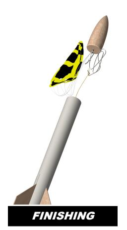
**20.** When all the fillets have dried, prepare balsa surfaces for a smooth professional looking finish. Round the edges of the fins, then fill the wood grain with balsa fillercoat or sanding sealer, When dry, sand with fine sandpaper. Repeat until smooth.
