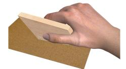
□ 4. Round all the edges of each fin, except the root edges. Leave them flat. Repeat for all four fins. The root edges will be glued to the body tube.
