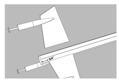
□ 20. Apply glue to the root edge of one of the triangular fins and position it along one of the lines drawn for the fins on the side of the body tube and even with the bottom of the main tube. Glue it using the same technique used on the main fins. Repeat for the other triangular fins. Allow the fins to completely dry, checking carefully to make sure they are parallel with the main body tube.
