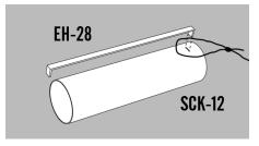
■ 8. Slide the centering ring without the slot (AR-2050) from the bottom of the engine tube until it is close to the slit in the engine tube and the Kevlar cord. Apply a bead of glue around both sides of the joint formed by the ring and tube, keeping glue off the outside edge of the ring. Tuck the free end of the Kevlar cord into the engine tube to keep it out of the way.
