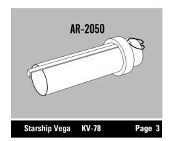
□ 9. Slide the Mylar retaining ring (HR-20) over the end of the engine tube until it is centered on the tube. Apply a bead of glue around both sides of the joint formed by the ring and tube, keeping glue off the engine hook end closest to the bottom of the engine tube.
