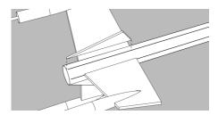
of one of the small fins and position it along one of the lines drawn for the main fins on the side of the body tube and 4-5/8" from the top of the main tube. Glue it using the same technique used on the main fins. Repeat for the other small fins. Allow the fins to completely dry, checking carefully to make sure they are parallel with the main body tube.
