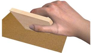
□ 4. Round all the edges of each fin, except the root edges. Leave them flat. Repeat for all four fins. The root edges will be glued to the body tube.
