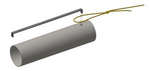
□ 9. Carefully remove the two centering rings from the laser-cut set (CR-7-55EH). Select the one with the small notch and align the notch over the engine hook, Slide it from the bottom of the engine tube until it is against the end of the engine hook and against the yellow Kevlar® cord.
