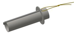
□ 10. Wrap masking tape around the center of the engine tube to hold the engine hook in place and centered along its length. Run a bead of glue over the masking tape and along the engine hook between the tape and the ring. Allow to dry.
