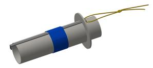
□ 11. Select the remaining centering ring that has the wider notch. Align the notch over the engine hook and slide it from the bottom of the engine tube until it is 1/2" from the bottom of the engine tube. Apply a bead of glue around both sides of both centering rings and against the engine tube. Keep glue away from the outer edges of both rings and from the notch in the lower ring. Make sure the engine hook moves freely. Allow to dry in an upright position.
