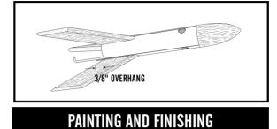
□ **13.** When the fillets have dried, prepare balsa suffaces for a smooth professional looking finish. Fill the wood grain with Fill'n'Finish diluted about half and half with water, When dry, sand with fine sandpaper. Repeat until smooth. Wipe off balsa dust.
