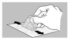
**4.** Sand a taper on each leading edge .21" wide and leave all the tip and root edges flat. For scale fins, sand to .05" thick.
