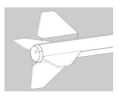
□ 16. After the fin assembly is completely dry, run a very small bead of glue along both sides of each fin-body tube joint. Using your forefinger, smooth the glue into fillets. Since this is a scale model, it should not have fillets showing. Wipe any excess glue and allow to dry.
