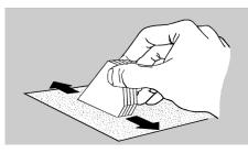
□ 3. Round the leading and trailing edges of each fin. Leave the tip and root edges flat. Repeat for all three fins. The trailing edge can be sanded to a bevel for a more aerodynamic shape. The root edge will be glued to the body tube.
