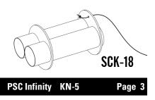
**9.** Insert an empty casing (**MC** -727) into one of the Sustainer engine mount tubes. Apply a bead of glue inside the sustainer body tube (**ST-16180**).
