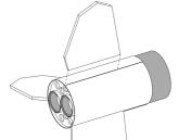
□ 23. After the fin assemblies are completely dry, run a small bead of glue along both sides of each fin-body tube joint. Using your forefinger, smooth the glue into fillets.
