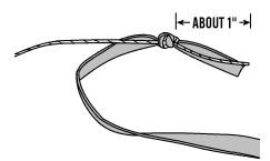
**26.** Tie the free end of the shock cord to the screw eye in the nose cone. Assemble the chute using the instructions supplied with the kit and attach to the screw eye as shown.
