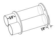
**7.** Apply a heavy fillet of glue around both sides of each centering ring at the joints with the engine mount tubes. Continue turning the assembly until the glue does not run. Set the assembly aside to dry completely.
