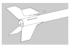
19. As the fins are drying, use the laser-cut fin template to align the fins perpendicular to the main body tube. The template will work with three or four fins. Turn it until the three fins line up with the corresponding slots. Do not let any glue set with the template in place.
