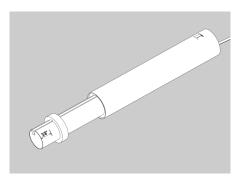
15. Pull the long end of the elastic cord taunt until the knot is seated against the top slit. Apply a bead of glue on the knot and on the part of the elastic cord that is exposed on the outside of the insulating tube. Wipe any excess glue from the outside of the insulating tube. Store the excess length of the elastic cord inside the insulating tube.
