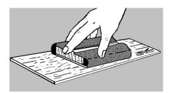
3. Stack all the fins in a group. Line the group up squarely and sand the fins back and forth over some fine sandpaper to get rid of the holdin tabs as shown below. Do not sand enough to change the shape of the fins.
