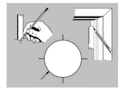
**23.** Place a mark on each line 3/8" from the end opposite the slit. Insert the engine hook in the slit.
