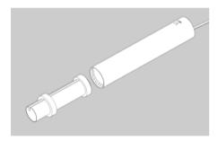
■ 14. Mark the engine mount 1/4" from the bottom of the engine tube.
