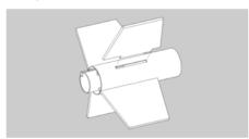
**29.** Apply a bead of glue inside the booster tube opposite the engine hook and insert the tube coupler (HTC-10) until just under 1/2" remains exposed.
