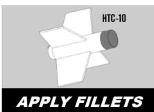
**30.** After the fin assembly is completely dry, run a small bead of glue along both sides of each finbody tube joint. Using your forefinger, smooth the glue into fillets. Apply a fillet of glue on each side of the launch lug. Allow this assembly to dry in a vertical position.
