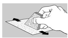
**4.** Round all the edges of each fin, except leave the root edges flat. Repeat for all six fins. The root edges will be glued to the body tube.
