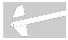
□ 12. Apply glue to the root edge of one of the long basswood fins and position it along one of the lines drawn for the fins on the side of the body tube and 1/4" from the top of
