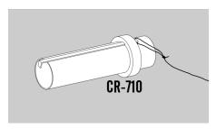
■ 8. Mark 1" from the bottom of the engine mount tube and slide the other centering ring (CR-710) from the bottom until it is even with the mark.
