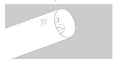
■ 16. Insert the insulating tube and engine mount assembly into the main body tube (ST-1083S3) until the lower centering ring is just outside the main body tube. Align the engine hook between two of the slots. Apply a heavy bead of glue around the top side of the lower centering ring.
