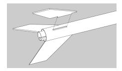
19. As the fins are drying, use the laser-cut fin template to align the fins perpendicular to the main body tube. The template will work with three or four fins. Turn it until the three fins line up with the corresponding slots. Do not let any glue set with the template in place.
