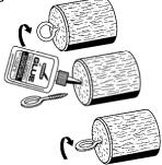
42. Check the nose block for fit. It may be necessary to sand it gently if the fit is too tight or build it up with masking tape if too loose. Mark the nose block 3/4" from one end. Apply glue to the inside the remaining body tube at a distance of 1/4" from one end.
