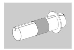
■ 10. Slide the centering ring with the long slot (CR-KD-4B) over the end of the engine tube. Space it about 1/16" from the bottom of the engine tube. Apply a bead of glue around both sides of the centering ring, keeping glue away from the engine hook and the notch.
