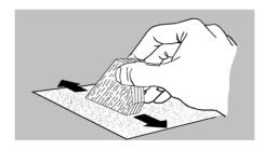
**4.** Sand a taper on each leading edge and trailing edge and leave all the tip and root edges flat.
