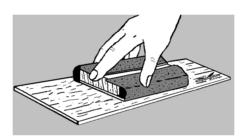
**3.** Stack all four fins in a group. Line the group up squarely and sand the fins back and forth over some fine sandpaper to get rid of the hold-in tabs as shown below. Sand the root edge *very gently*.
