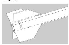
**20.** After the fin assembly is completely dry, run a very small bead of glue along both sides of each fin-body tube joint. Using your forefinger, smooth the glue into fillets. Since this is a scale model, it should not have fillets showing. Wipe any excess glue and allow to dry.
