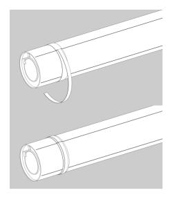
**18.** Apply a very thin bead of glue to the dull side of the other band on the widest half. Starting the wide end on the same marked fin line as the lower band, and even with the top of the body tube, apply the band the same as the lower band.
