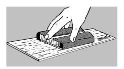
**□ 3.** Stack all the fins in a group. Line the group up squarely and sand the fins back and forth over some fine sandpaper to get rid of the hold-in tabs as shown below. Do not sand enough to change the shape of the fins.
