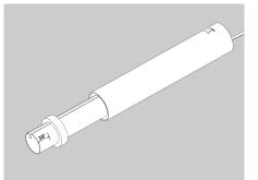
☐ 15. Pull the long end of the elastic cord taunt until the knot is seated against the top slit. Apply a bead of glue on the knot and on the part of the elastic cord that is exposed on the outside of the insulating tube. Wipe any excess glue from the outside of the insulating tube. Store the excess length of the elastic cord inside the insulating tube.
