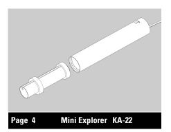
**14.** Mark the engine mount 3/8" from the bottom of the engine tube.
