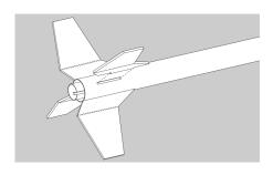
**22.** As the fins are drying, use the laser-cut fin template to align the fins perpendicular to the main body tube. The template will work with three or four fins. Turn it until the four fins line up with the corresponding slots. Do not let any glue set with the template in place.
