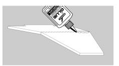
**7.** Round all the edges except the root edges of each fin. Do not sand the root edge or the tab will not contact the engine tube in a later step.
