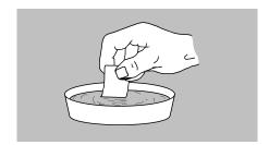
**34.** Slide the decal in place and use the paper backing to work the bubbles out. Repeat for all the decals.
