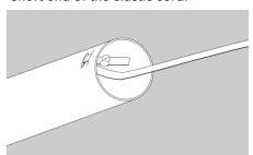
□ 16. Apply a bead of glue inside the bottom of the insulating tube (away from the elastic cord.) Insert the engine mount into the insulating tube until it is recessed about 1/16". Roll the assembly on a flat surface to make sure it is aligned properly.
