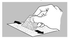
Made in two interlocking pieces for added strength. Using a piece of wax paper, align the first set as shown. The two pieces will only fit well if they are oriented correctly. Apply a bead of glue along the wavy edge of the smaller piece. Test fit the two pieces together to get glue on both edges. Pull them apart and allow to dry for a few minutes. Repeat for the other three sets. Allow the glue to get tacky for the next step. Do not allow them to dry completely.
