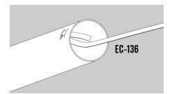
**15.** Tie an overhand knot in the short end of the elastic cord.
