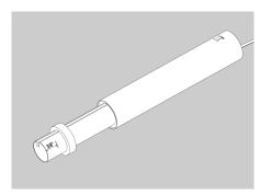
■ 18. Pull the long end of the elastic cord taunt until the knot is seated against the top slit. Apply a bead of glue on the knot and on the part of the elastic cord that is exposed on the outside of the insulating tube. Wipe any excess glue from the outside of the insulating tube. Store the excess length of the elastic cord inside the insulating tube.
