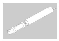
17. Mark the engine mount 3/8" from the bottom of the engine tube.
