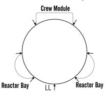
□ 18. Using the same channel, mark the long reactor bay tube (BT-5SE) at the two small laser-cut marks between the two slots. Using a sharp hobby knife, cut the tube into two identical halves along the marked lines
