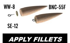
□ **39.** After all joints are completely dry, run a small bead of glue along both sides of each fin-body tube joint, the launch lug assemblies and the reactor tube assemblies. Using your forefinger, smooth the glue into fillets. Apply a fillet of glue on each side of the launch lugs. Allow this assembly to dry in a vertical position.
