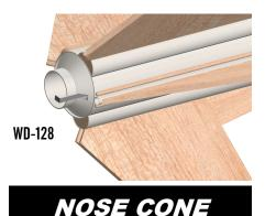
**37.** Insert the nose cone (**BNC-55F**) in the main body tube and check for proper fit. The nose cone should be snug to hold itself in alignment. If it is too loose, add masking tape. If it is too tight, sand the shoulder slightly.
